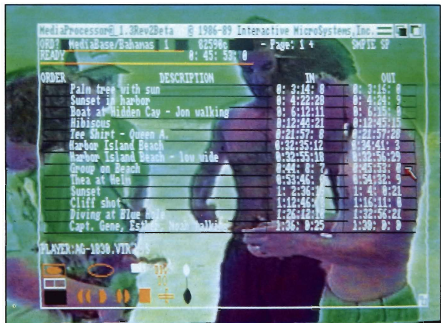
Overlays are easily accomplished by use of a genlock
